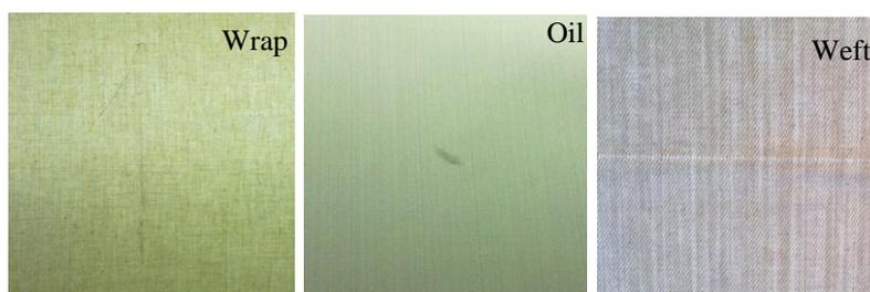
Fig. 10 Wrap, Oil and Weft faulty fabric images in size 256x256 px
